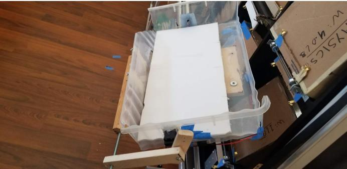
Figure D 4: Tray Mounted on Railing Tracks (sliders) [52]
