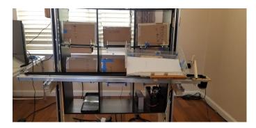
Figure 2: Rail system with stepper motors and tray [26]
