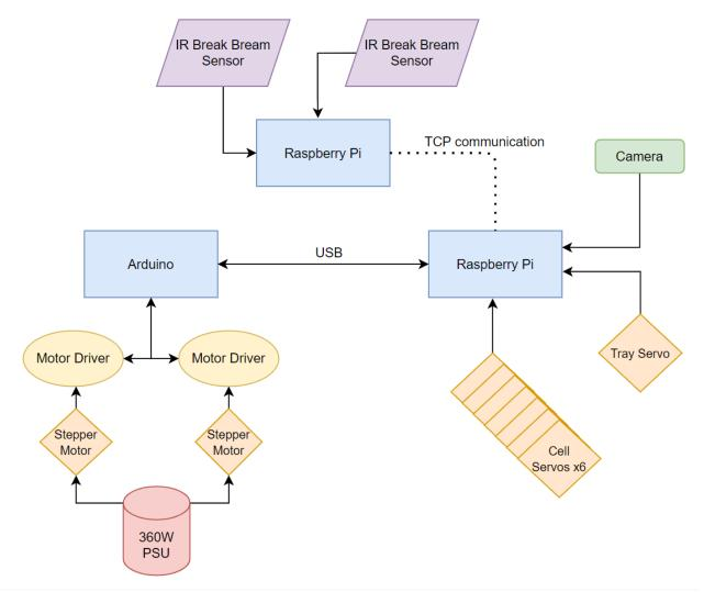
Figure B 1: Large-Scale Machine Hardware Block Diagram
