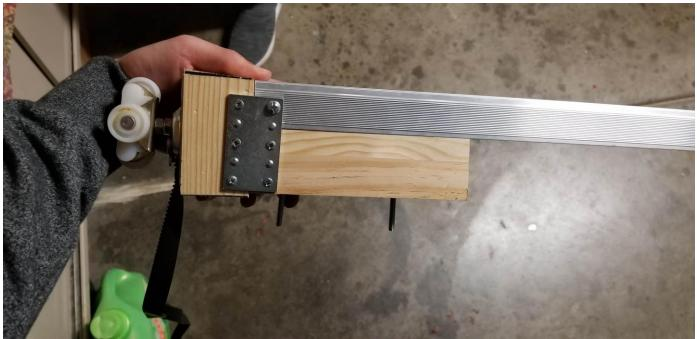
Figure D 6: Mount used to hold Horizontal slider with Vertical slider [52]
